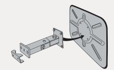
> All stainless steel mirrors are supplied with fully adjustable bolts and galvanised steel bracket kit for wall or round steel posts (Ø76 to 90mm) or rectangular steel posts (60x80mm or 80x80mm)
