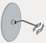
> The mirror is mounted on an articulated ball joint, supplied with wall or post mounting kit
